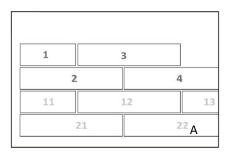
A. Products should be staggered in brick laid pattern, stagger equal to half of a plank for the first 2 rows, and then at least 18" for the following rows. Spacers should be placed against walls to maintain proper distance (1/4" - 1/2"). Tools needed: planks, underlayment, spacers
